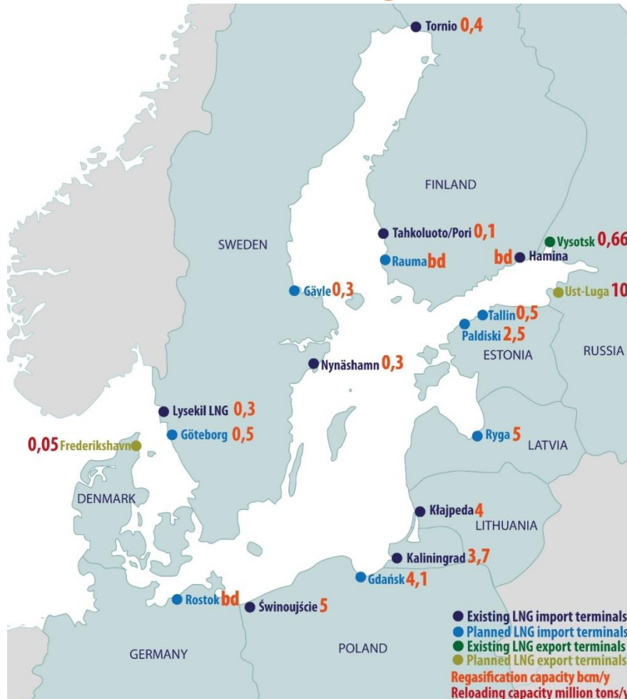
LNG terminals in the Baltic Sea region (existing and planned) Source: prepared by Actia Forum
