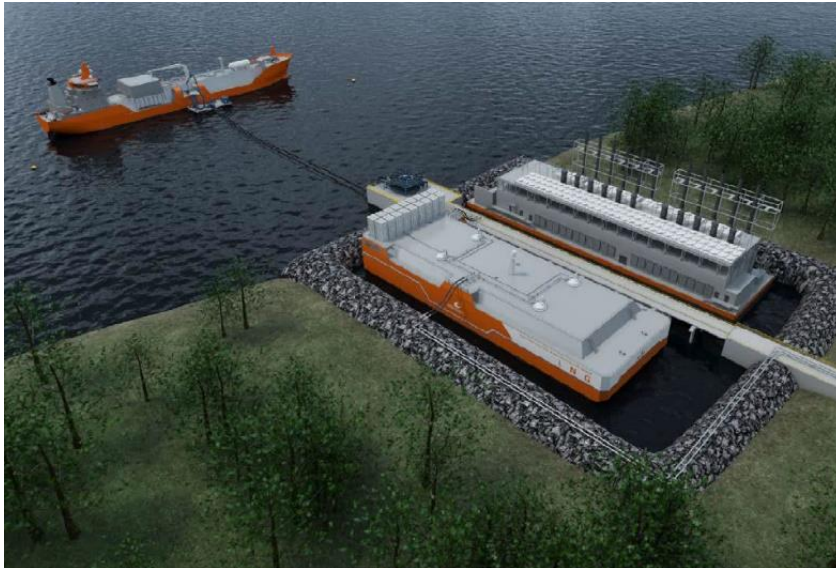
Example visualization of LNG storage and regasification barge and LNG vessel during unloading Source: Wärtsilä
